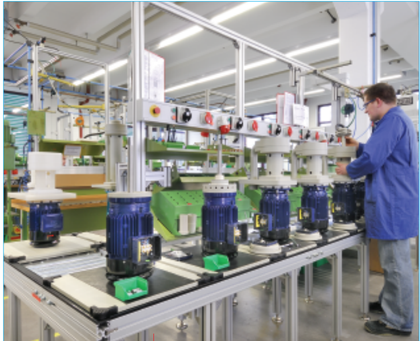
Manual work is required in the final assembly stage, with experienced staff assembling components to make high-precision units
